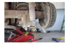
Remove the 10 bolts (½") securing the axel cover. Make sure to have something below the axle to catch the Differential fluid. The axle should contain about two quarts of fluid. While the fluid is draining, scrape off all of the old gasket and silicon from the pumpkin and cover. I also painted the brackets purchased from North Cobra and the pumpkin cover. I painted them with high temp gray paint. You can choose any paint color, but I recommend using high temp paint.
