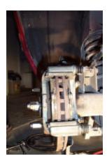
You should now have the brakes installed with exception of the brake lines and Emergency Brake cables.
